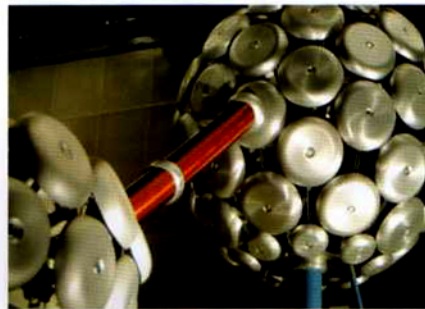
BTU Cottbus high voltage test equipment
